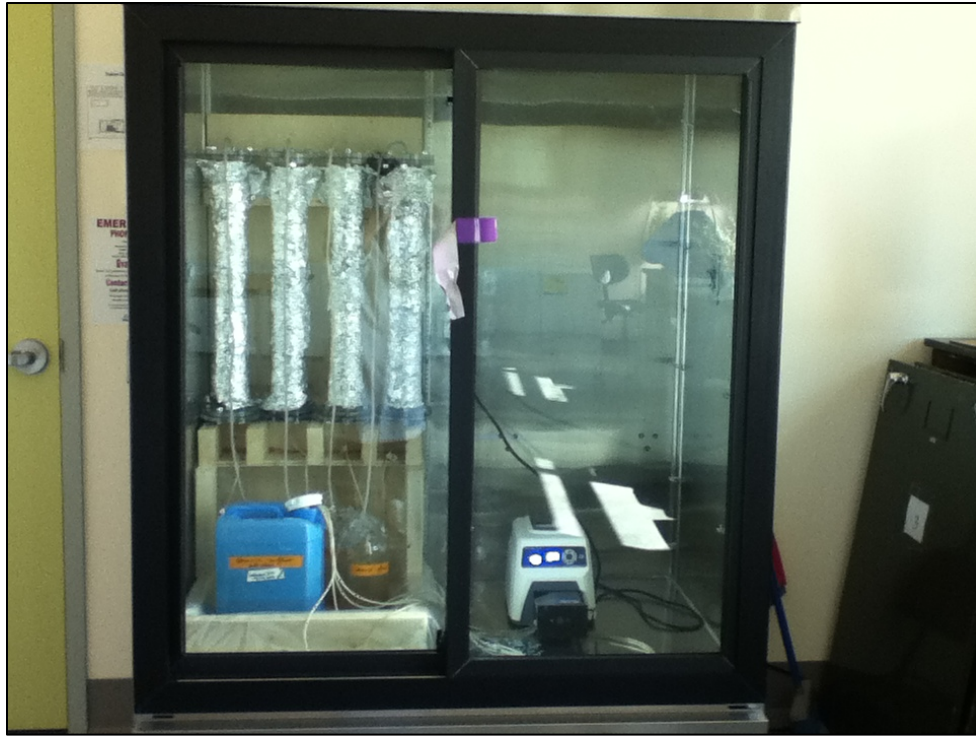
Figure 5. Operation of the C9 to C12 bioreactors in the laboratory fridge at 6°C
