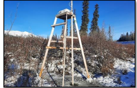
Figure 2. Wood tripod with SIMBA unit installed at the top.
