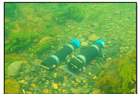
Figure 1. A pair of anchored plates at the bed of a stream to which the aquatic sensors are attached.
