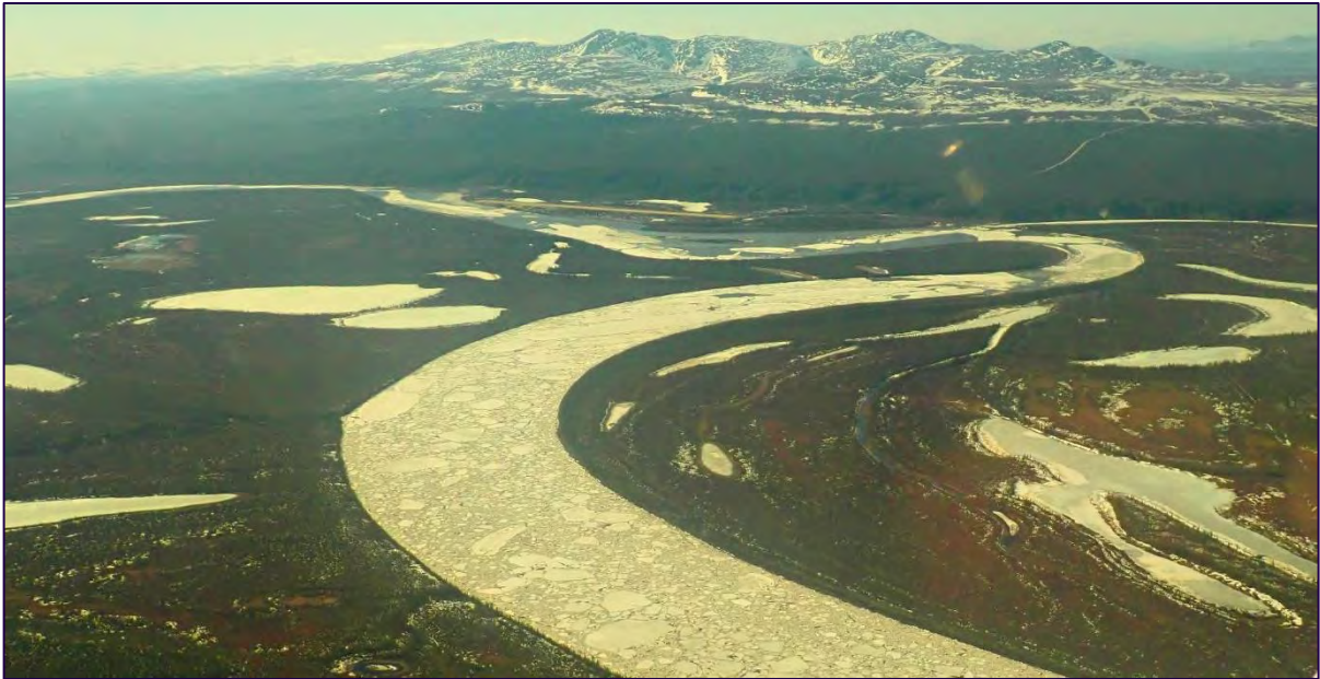
FIGURE 6.4.5. TOE AREA OF THE ICE JAM UPSTREAM OF OLD CROW ON MAY 12 AT ABOUT 5:15 PM. THE OLD CROW AIRSTRIP IS VISIBLE IN THE BACKGROUND (LOOKING NORTHWEST).
