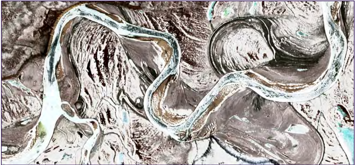
FIGURE 6.4.2. COPERNICUS SENTINEL-2 IMAGE (TRUE COLOUR) FOR MAY 8, 2020, SHOWING KM 343 TO 362 OF THE PORCUPINE RIVER. THE BLUEFISH RIVER AUFEIS APPEARS INTACT WHEREAS THE UPSTREAM ICE COVER (ON THE RIGHT) IS BECOMING EXPOSED TO SHORTWAVE RADIATION.
