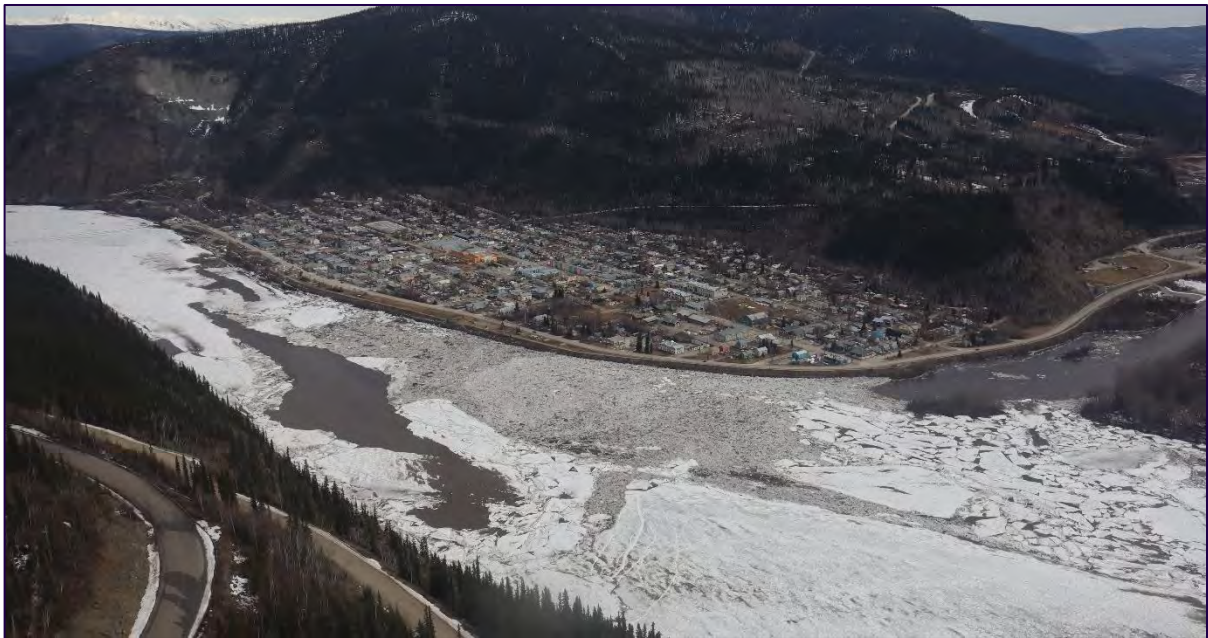
FIGURE 6.4.4. TOE OF A COMBINED KLONDIKE RIVER (DARKER) AND YUKON RIVER (LARGER ICE SLABS) ICE JAM AT DAWSON ON MAY 9, 2023, AROUND 2 PM.
